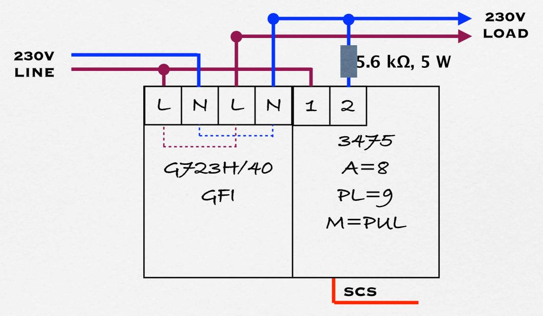
GFI = GROUND FAULT INTERRUPTER, MEASURES THE DIFFERENCE BETWEEN THE CURRENTS IN THE LINE AND RETURN WIRES.
